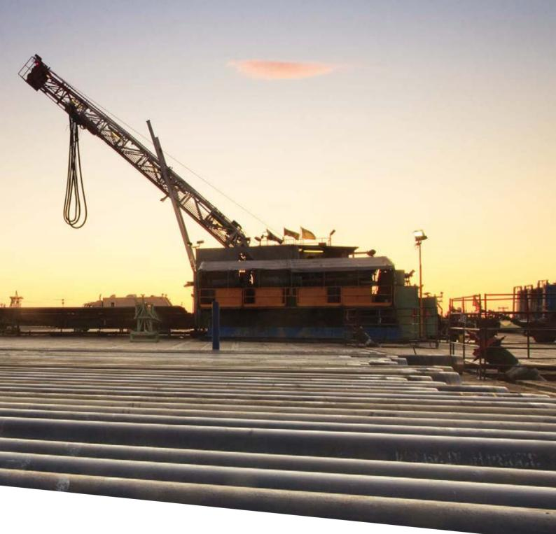
Alberta, utilises an *in situ* technique that employs steam-assisted gravity drainage techniques (SAGD), coupled with horizontal drilling methods, to extract the bitumen.
